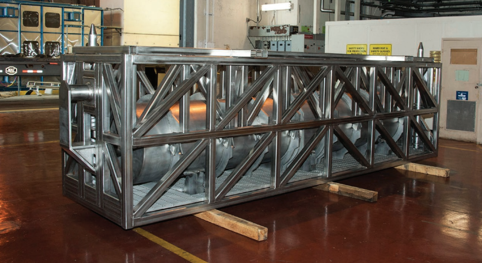
A cask for carrying MK-18 targets. photo: Savannah River Site Photography
