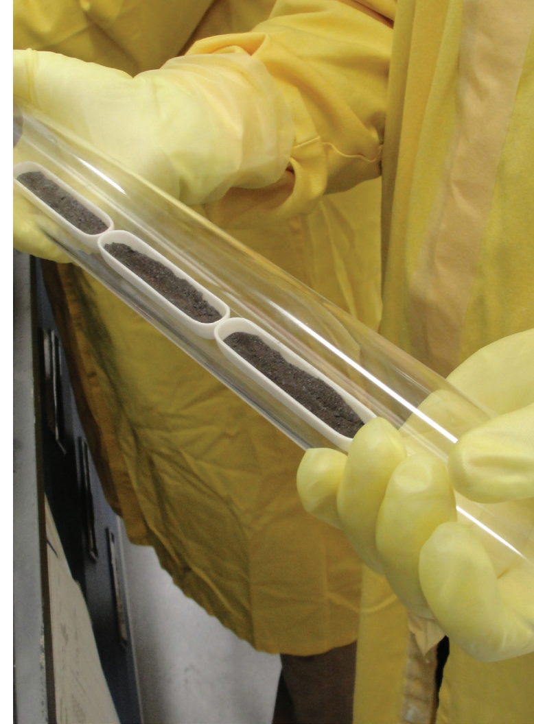
Loaded crucibles in a process tube prior to insertion into the tube furnace. (Photo: Bryan Foley, SRNL)
