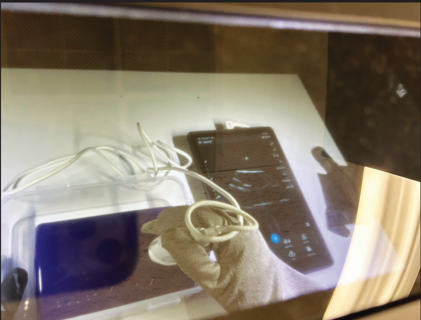
A device is tested in an environment with no external communication interference (Photo: Mitchell Jordan)
