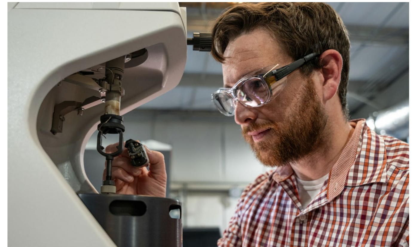
Cam Chatham loads a sample of a new material developed for additive manufacturing into the dynamic mechanical analyzer (DMA).
