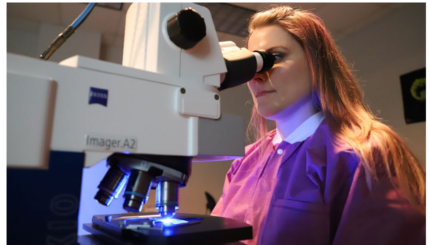
Courtney Burckhalter is using an epifluorescence microscope to search for signs of Legionella pneumophila. Samples are regularly taken and analyzed for signs of Legionella pneumophila or the conditions conducive to the bacteria’s growth. SRNL photo by Chris O’Neil, APR.
