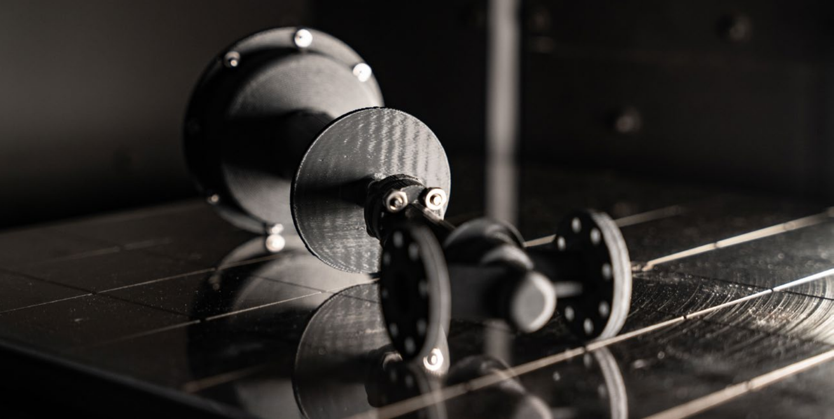
A 3D printed automated chilled water valve sits inside a printer in SRNL's Applied Additive Manufacturing Lab. The part was printed on the model 450 printer in high resolution ASA material.
