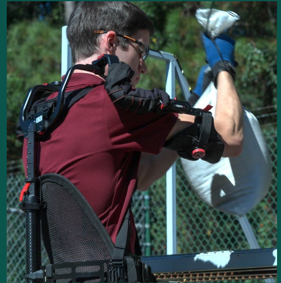
The shoulderX device reduces shoulder strain and fatigue associated with overhead lifting.
