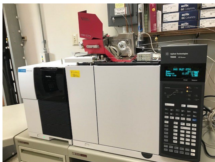
Figure 1. A gas chromatography – mass spectrometry (GC-MS) instrument for analyzing air or liquid samples.
