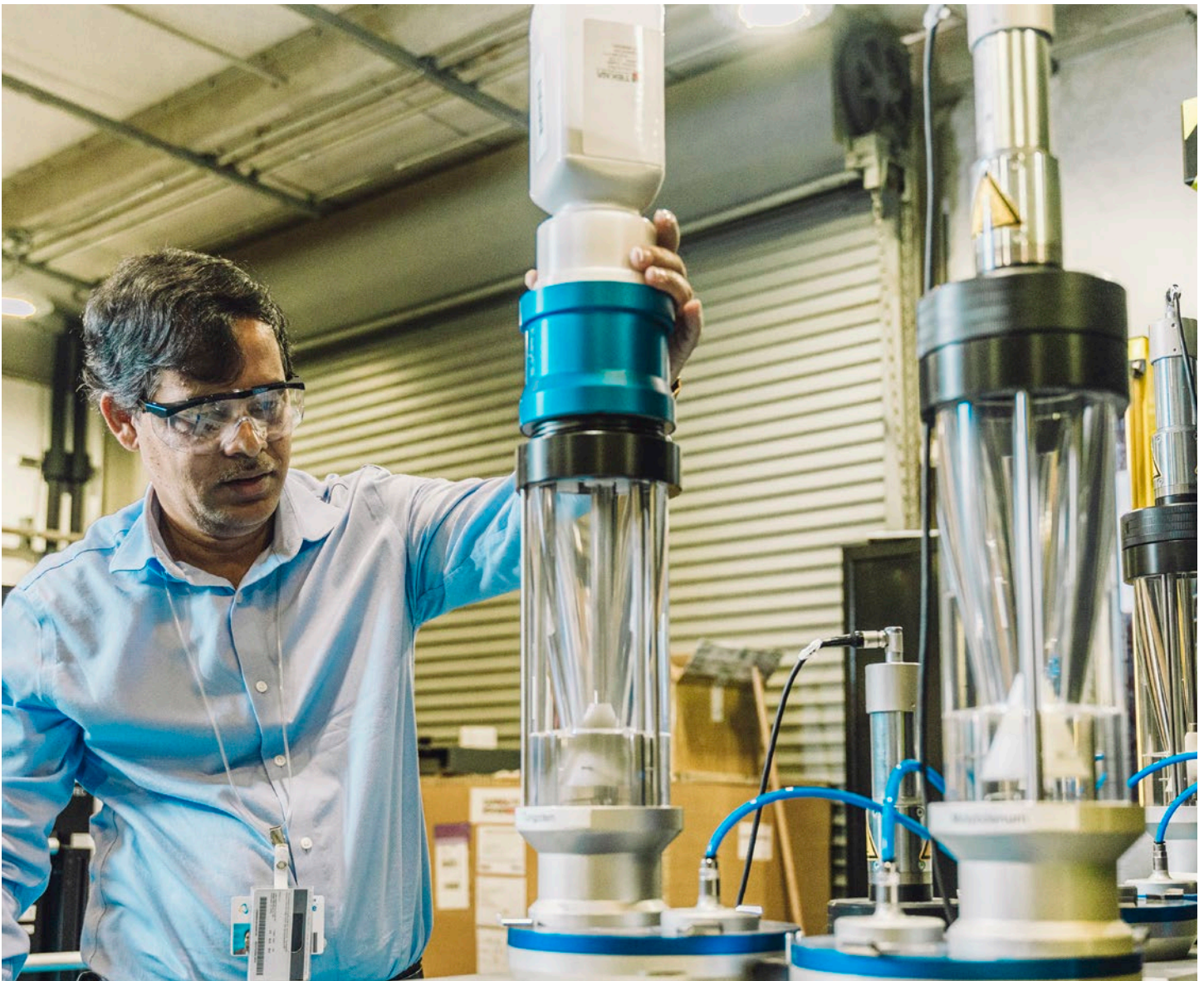
The powder feeders are filled with different metal powders to create an alloy.
