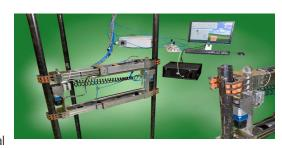
pipes, maintaining a constant grip by one arm while swinging into position for a stronghold by the other arm. The flexible and extendable arms of the Orangutank<sup>TM</sup> allows for variances in pipe spacing and configurations.
