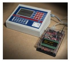
devices securely and at low-cost due to operating system free embedded microprocessors. With input types to include digital data streams, voltage levels, 4-20mA, RTDs and thermocouples, and various others, this device has uses in any field requiring data sharing in "business sensitive" or agency oversight applications such as process or material monitors, electrical power grid data sharing and usage, network backbone throughput and cost-sharing data sources.
