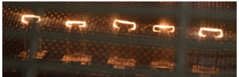
Photo of RGO filaments heated to ~ 1400 C; alternative filament assemblies used for this photo
