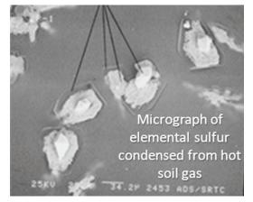
an improved remediation method to distribute elemental sulfur into contaminated soil to treat elemental mercury. Elemental mercury reacts with the sulfur to form stable compounds with low solubility and low toxicity. Because gases move easily in soil, gaseous delivery of a chemical reagent is a preferred enhancement for many in situ treatment processes.
