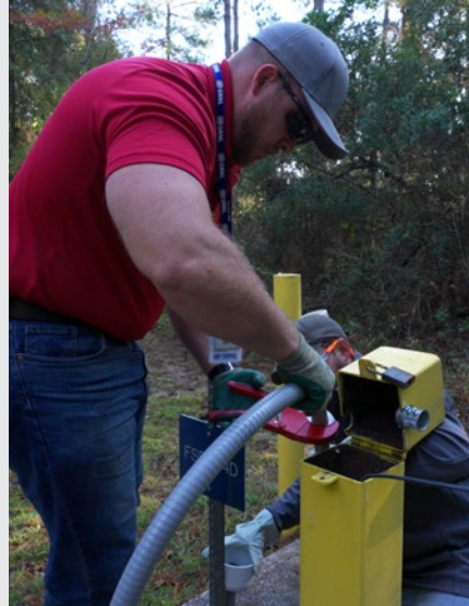
SRNL Scientists installing an ALTEMIS well monitor at the Savannah River Site
