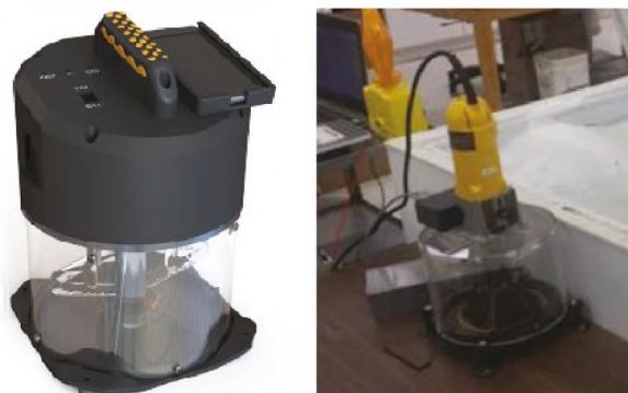
**Figure 1:** TMFD Conceptual(left) and Prototype (Right) Device.
