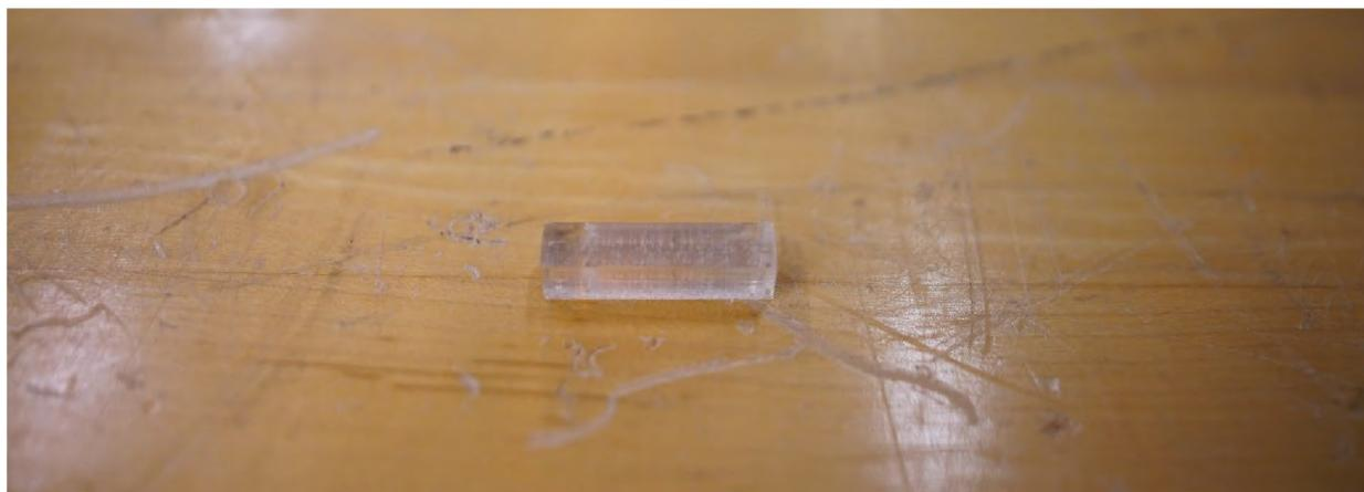
**Figure 5:** Unpolished 10% PETG/ 90% PC Mixture printed at 20 micron layer height.
