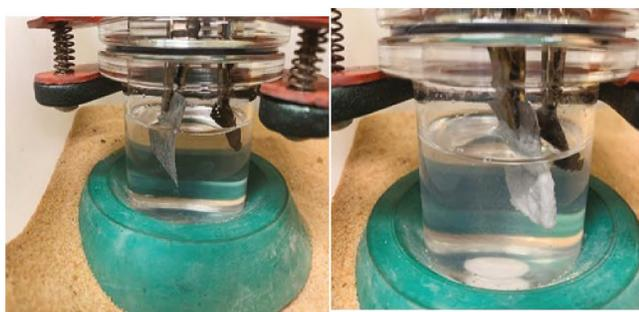
Figure 4: Show no TEDA:AlH<sub>3</sub> before applying voltage and the formation TADA:AlH<sub>3</sub> when voltage is applied.
