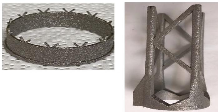
**Figure 3:** 3D/4D printed metal hydride objects.
