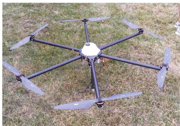
Figure 2: Hexacopter fabricated by VA Tech's Unmanned Systems Lab.
