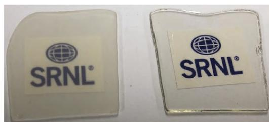
**Figure 2:** Low (left) and high (right) polish unirradiated glass cross section specimens.
