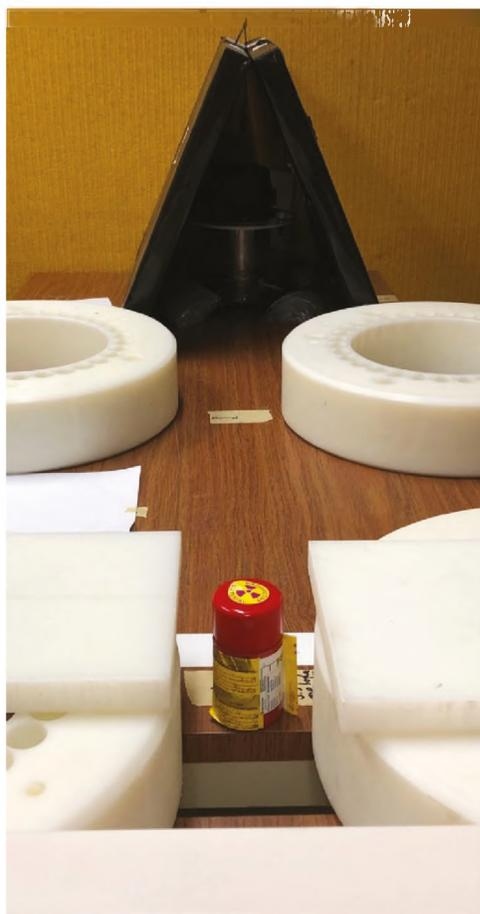
**Figure 6:** SRNL TMFD neutron irradiation set-up.
