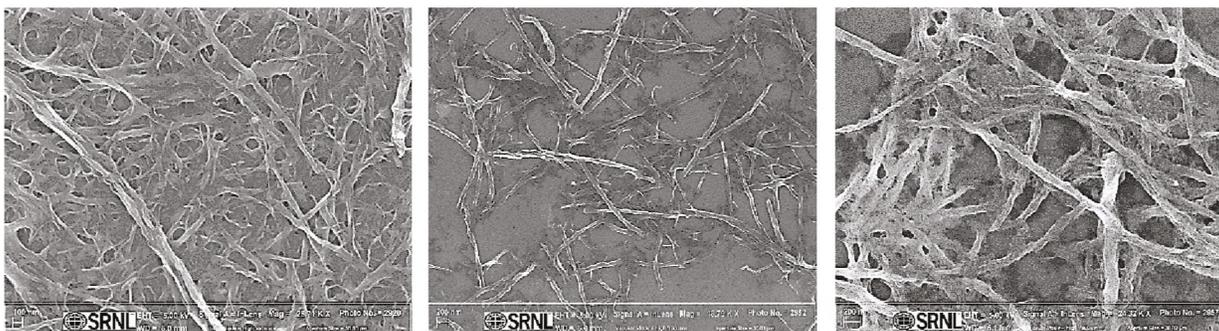
**Figure 6:** Examples of GONRs synthesized by three different syntheses based on the Hummer's method. These GONRs have 32 to 38 % oxygen functionality, form stable aqueous suspensions and are expected to provide better cement paste reinforcement than PUCNTs based on morphology and high aspect ratio.
