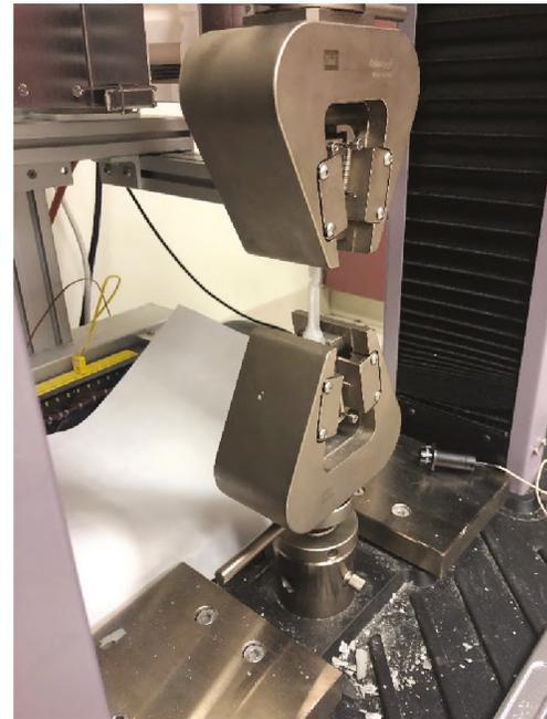
Figure 1: Tensile testing of dog bone samples.
