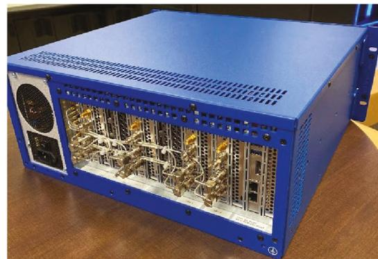
Figure 1: BroadSim NAVWAR GNSS simulator.
