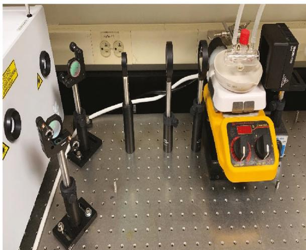
**Figure 1:** Optical setup. Pathway: laser tuner, turning mirrors, Galilean beam expander, beam focuser, sample cell, beam dump.
